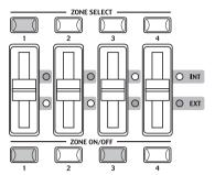
When the multitimbre is off, the default settings of the zones are as follows. It is recomended for simple MIDI transmit/receive use on stage etc. The default TXchannel is System Ch (see page45).
